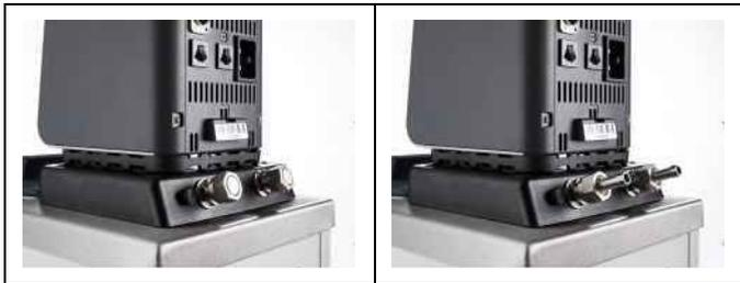
1. Remove the union nuts on the pump connections.
