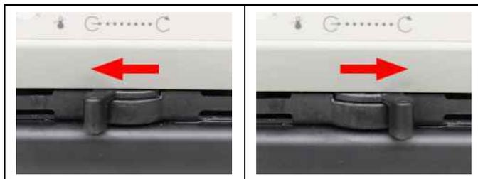
1. Set the lever to a low level for internal circulation (e.g. position 2 from the right stop).
