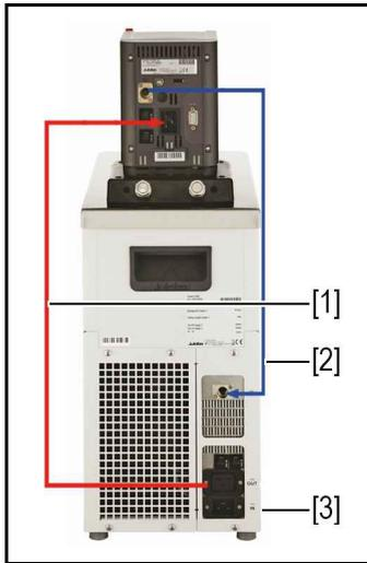
1. Connect the connection cable [1] of the circulator with the refrigeration unit.
