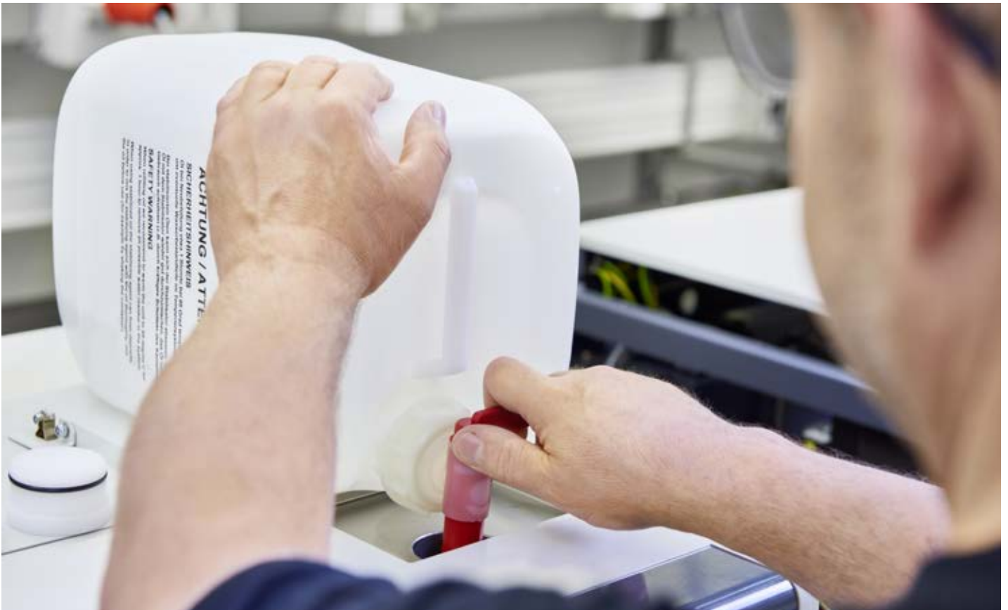
The filling port should be located so that filling is as easy and clean as possible and no spilled fluid enters the unit.
