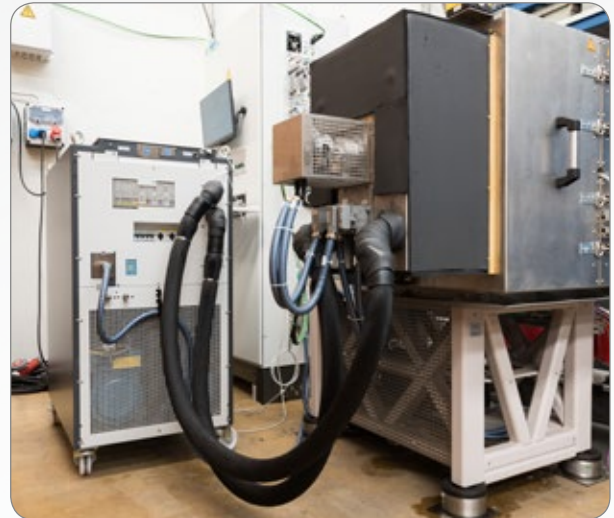
Fig. 8: Universal test chamber, where test specimens are exposed to simulated ambient and extreme temperatures
