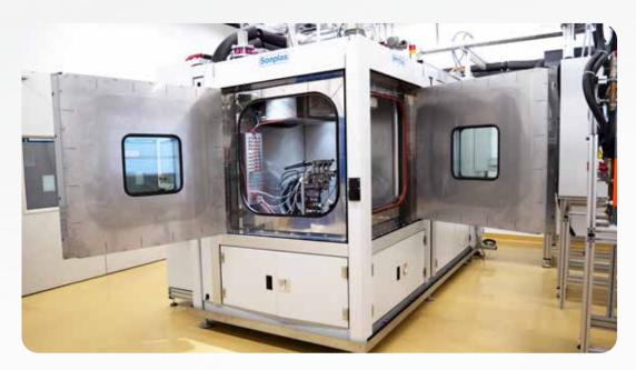
This concept, combined with further measures regarding explosion protection, predestines the Sonplas thermal chambers for testing of products where a release of explosive substances can be expected. This may be the case when using conventional, biological or synthetic fuels as well as hydrogen, methane or other explosive gases and mixtures, for example from batteries.
