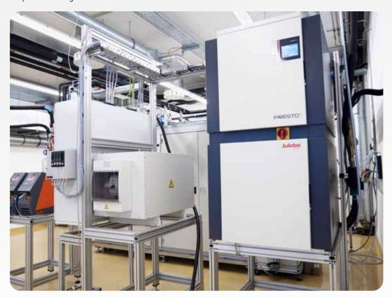
In addition, the units in the PRESTO W91 series offer sufficient power reserve to be able to operate, in special cases, in a temperature range of down to -91  $^{\circ}$ C minimum temperature and up to +250  $^{\circ}$ C maximum temperature.
