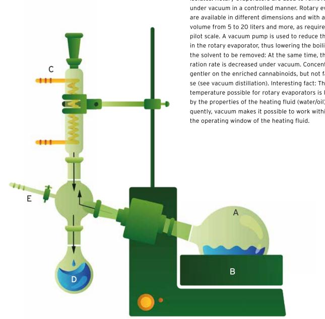
Flow of evaporation process during rotary evaporation
