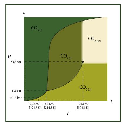
Fig. 1: Phase diagram of carbon dioxide
