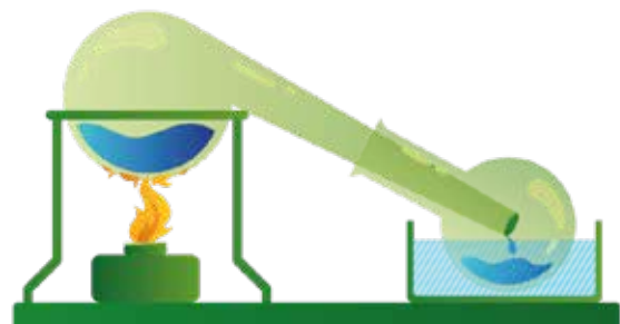
Overhead distillation: This is a simple distillative separation method for liquid mixtures.
