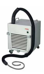
Moreover, most vacuum pumps are equipped with a cold trap on top because of this. In this cold trap, volatile components penetrating into the main condenser are separated at -40°C to -90°C so that they do not reach the pump. An immersion cooler, such as a Julabo FT-200 or FT-900, is suitable for controlling the cold trap.
