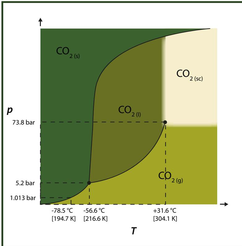
Fig. 1: Phase diagram of carbon dioxide
