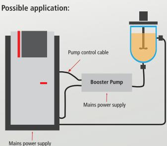
The Mag Drive Booster Pump can increase your fluid pressure up to 2.1 bar. The stainless steel design of the Pump provides excellent resistivity against chemical effects.
