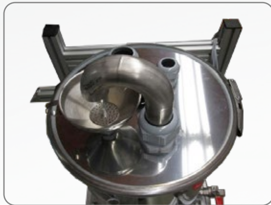
Technical refinements such as a filter at the inlet reduce the entry of dirt into the overall system and thus reduce, among other things, maintenance intervals and fluid changes
