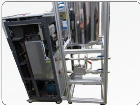
The special rack with additional tank connected to the PRESTO
